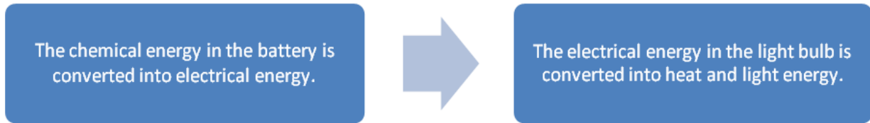
Figure 1. Energy conversion in a simple electrical circuit.
